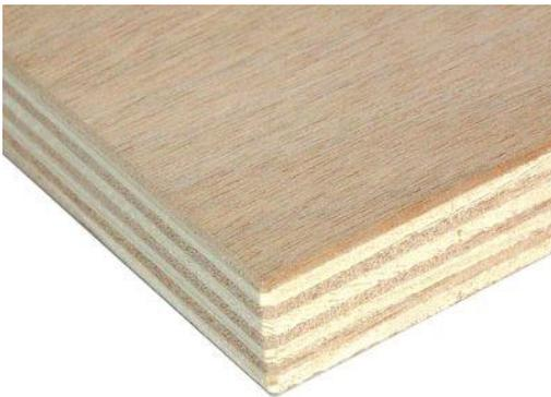
Plywood is a sheet material manufactured from thin layers or "plies" of wood veneer that are glued together with adjacent layers having their wood grain rotated up to 90 degrees to one another. Plywood was designed to compensate for some of the inherent weaknesses in wood products. Each layer of plywood is laid with the grain turned in such a way that it reinforces the weak spots of the other layer. This creates a wood panel that is incredibly strong and durable.
